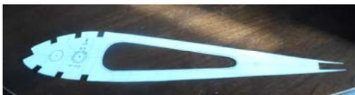
Once the pattern was established, a block of balsa suitable to provide all needed ribs was acquired and shaped as well as sliced.
